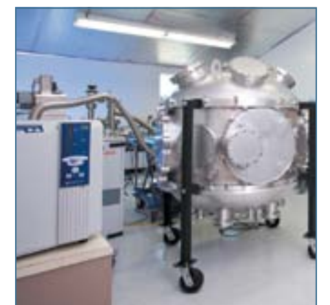
Helium mass spectrometer leak testing and RGA underway in our QC department.
