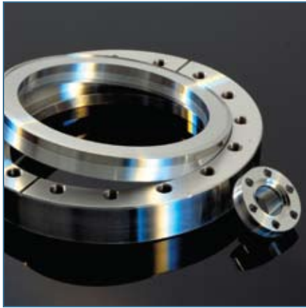
Atlas bimetallic CF flanges—the aluminum flange with a stainless steel knife-edge seal, make UHV aluminum vacuum systems a reality.
