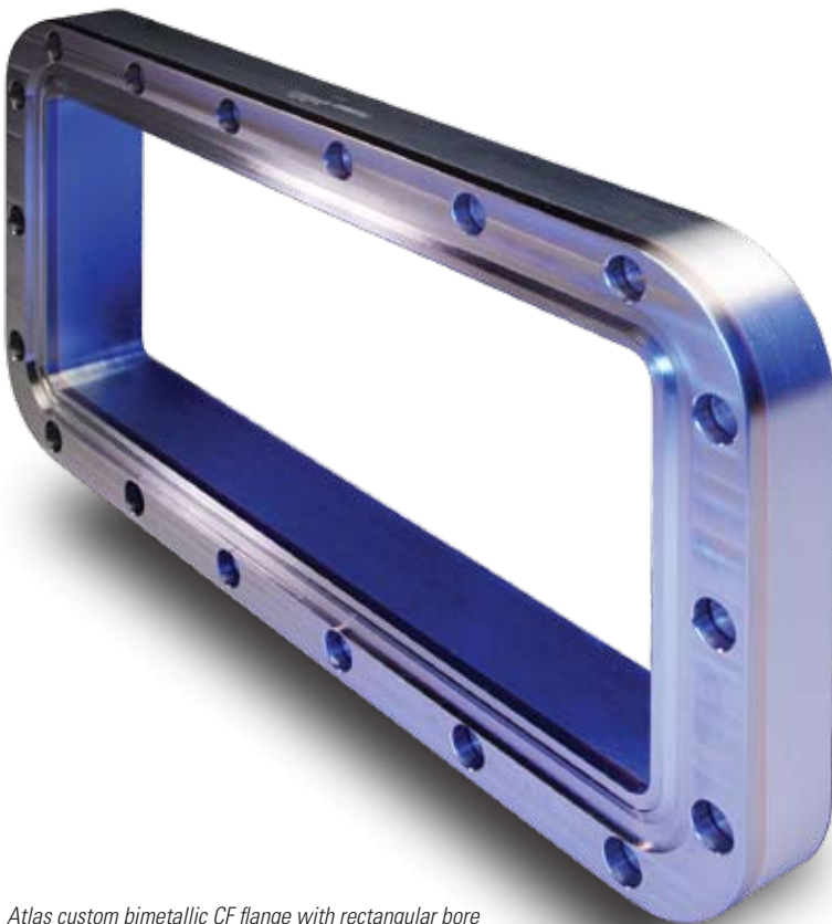
Atlas custom bimetallic CF flange with rectangular bore and knife-edge geometry provide maximum aperture and flexibility in UHV box-chamber applications.
