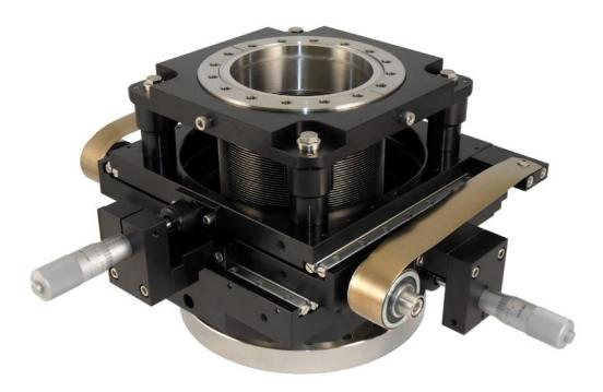
To make your selection, add the total travel required in either the X or Y axis to the **maximum** diameter of the device that will pass through the **HOMC3000**. This sum determines the *minimum* bellows inside diameter (ID).
