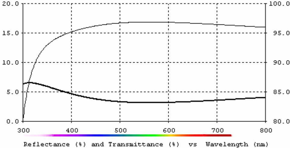
More complex multi-layer dielectric coatings enable a wide variety of tailored transmission / reflection characteristics giving for example virtually zero reflection at a single design wavelength ('V' coating) or at two wavelengths ('W' coating), or over a wide band BBAR or a neutral density attenuation, and many others.
