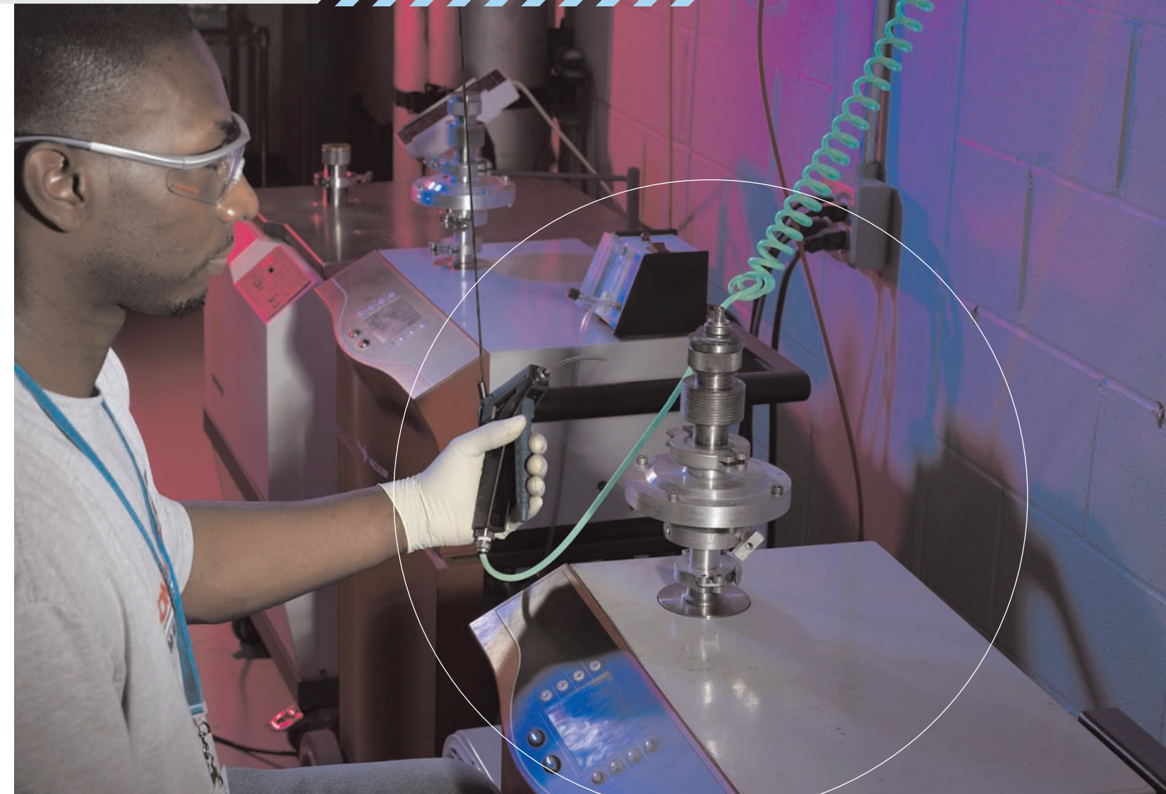
Helium leak testing of our Ceramaseal® products.
