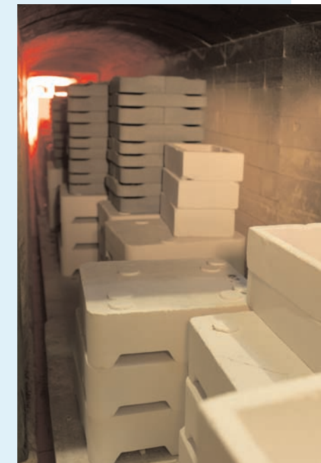
Continuous tunnel kiln used to fire ceramic insulators.
