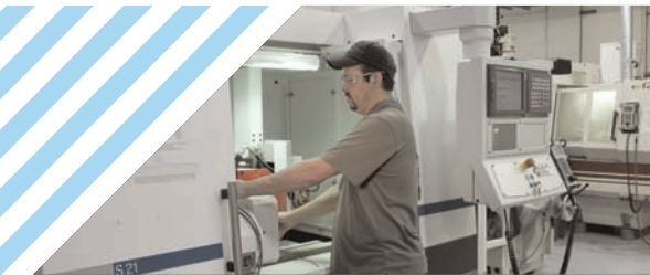
Hard (diamond) grinding of ceramic products to achieve tight tolerances.
